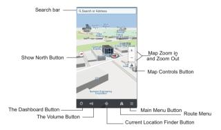
Map Controls button . Tap the button once to open the map controls dialog. It has toggles to switch between a two-dimensional (aerial) map view and a three dimensional (depth-perspective) map view. It also contains toggles for live traffic, day/night map theme and 3D terrain view
