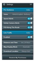
**Pro Guidance :** Pro Guidance enables Turn-by-turn Voice Instructions, Automatic Rerouting, Speed Alerts, Lane Assistance and POI Along the Route Features.
